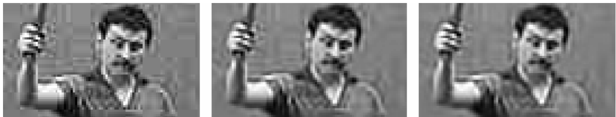
Figure 6. Left: MPEG-compressed Tennis video frame at PSNR of 24.32 dB Center: Deblocked image using proposed algorithm Right: Deblocked image using original Nosratinia algorithm
