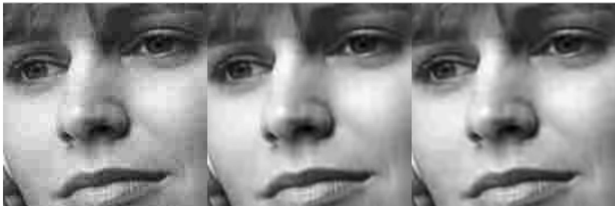
Figure 5. Left: MPEG-compressed Susi video frame at PSNR of 24.32 dB Center: Deblocked image using proposed algorithm Right: Deblocked image using original Nosratinia algorithm
